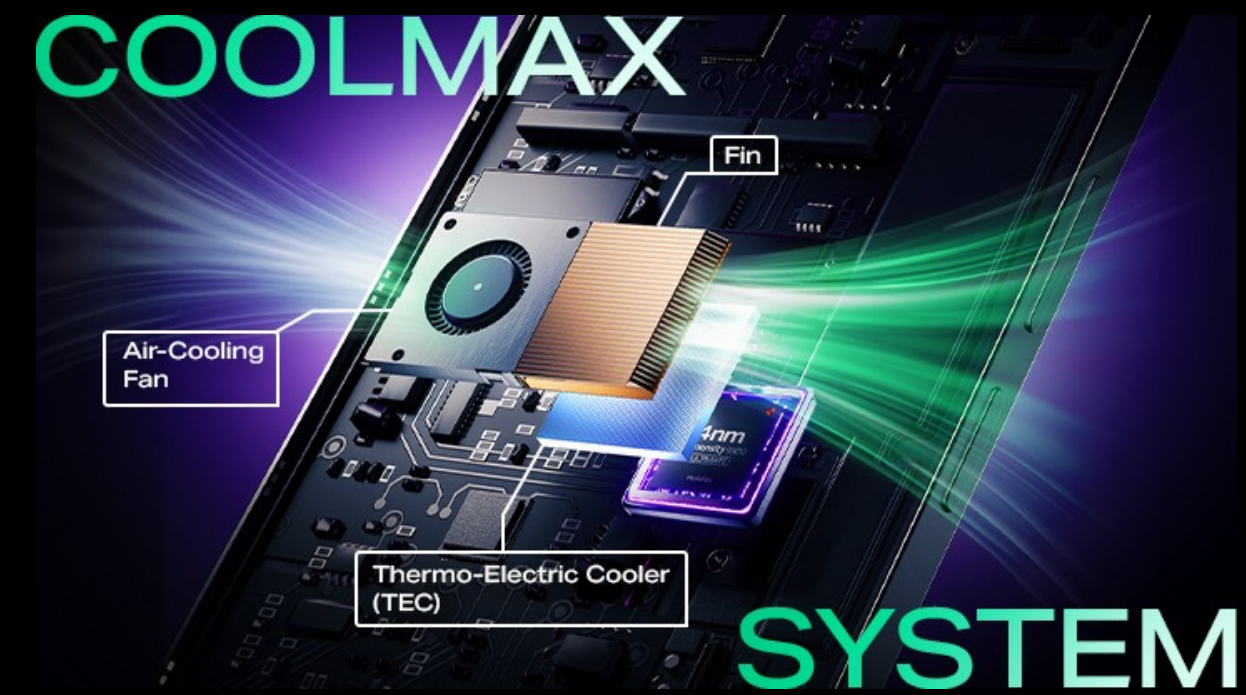
Industry-First Hybrid Cooling System: Semiconductor + Air-Cooling
